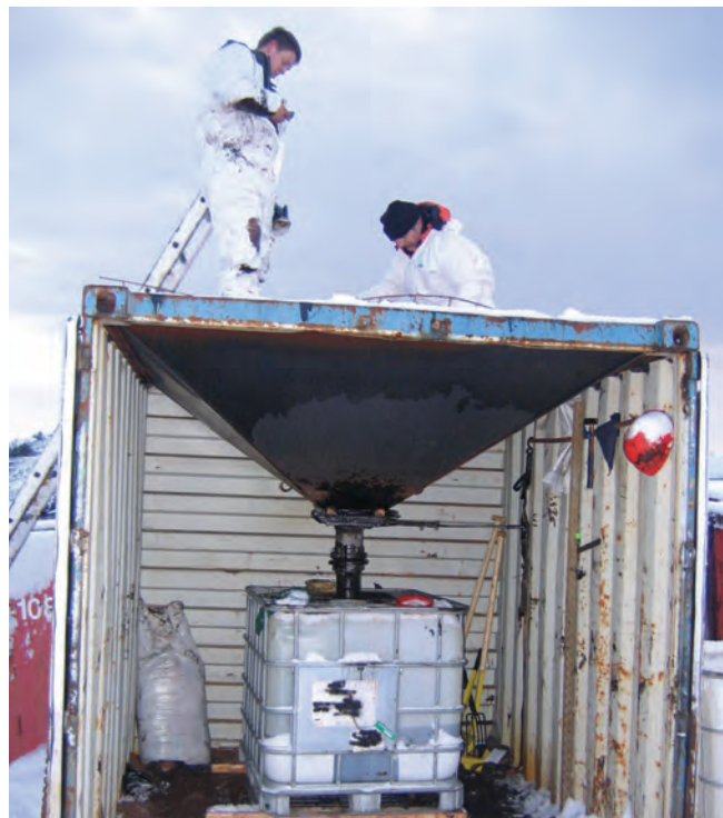
▲ Figure 16: An improvised waste filtration system, where recovered oil is passed through a grilled funnel to filter out debris.
