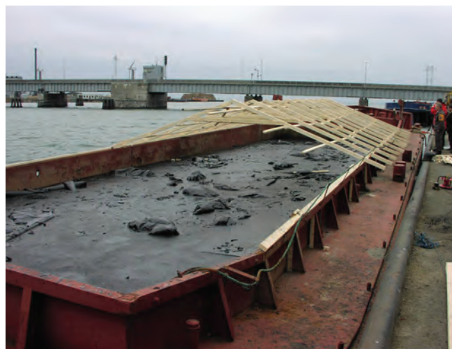
▲ Figure 10: Recovered oil stored in a barge. A cover is required to prevent rainwater ingress.
