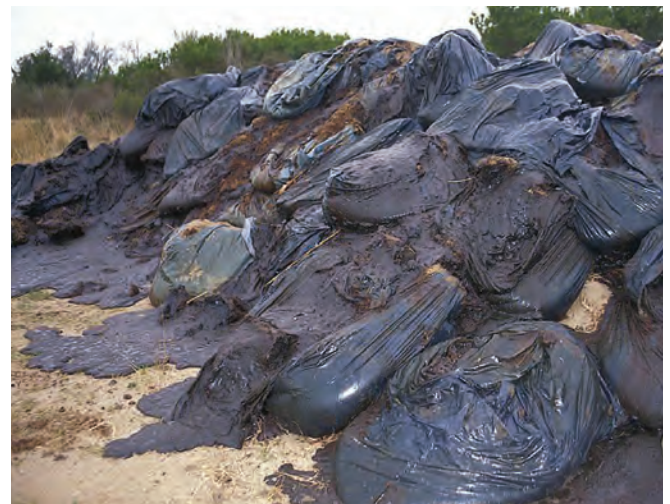
▲ Figure 12: Degradation of plastic sacks by long-term exposure to sunlight can lead to recontamination.
